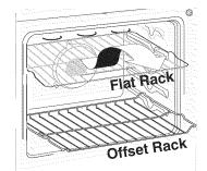
The **Offset Oven Rack** is used to maximize cooking space. The offset rack can be used in the lowest rack position to roast large cuts of meat and poultry or for specific type of cooking as per the table below.
